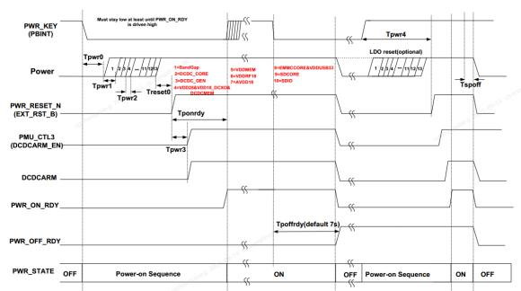
Integrated 7s reset circuit supports below two mode by SW select
