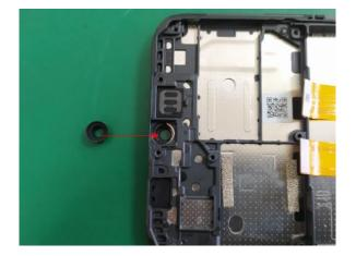
Assemble the receiver in the front assy.
