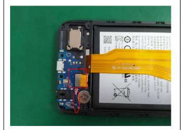
10 Assemble the SUB PCBA cover to SUB PCBA.
