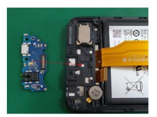
8 Assemble the RF cable to SUB PCBA.
